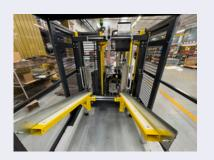
Gravity in-line magazine with storage capacity of up to 150 boxes, aligned with the box erection path to minimize the overall machine footprint—ideal where space saving is crucial.
