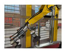
It is equipped with an arm activated by a pneumatic (Venturi) system and suction cups, used to pick cartons from the box storage, fold them, and transfer them via drive belts for bottom flap folding and sealing.
