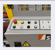
Simple integrated control panel equipped with different features: Manual mode, Automatic mode, Emergency, Reset, Start
