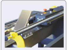
Easy and safe bottom flap folding system combined with tubolar pneumatic centering system, that holds the boxes in vertical to proceed with product filling and final sealing
