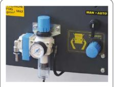
With a selector it is possible to work in both manual and automatic operations increasing the speed performance
