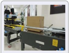
According to the different semi-auto case sealer in SIAT range, dedicated fixing plates are available to integrate F105 to create a complete packing station
