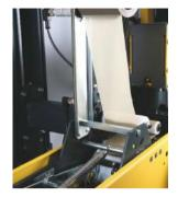
Fast unit changeover, height adjustment by handles, mechanical micro switch for lenght management and ON-OFF main eletrical switch for an easy and fast start up
