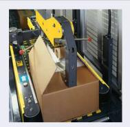
Easy setting pneumatic kicker combined with mechanical passive side flap folder to automatically close 4 top flaps without operator need
